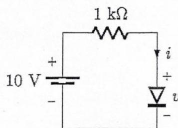
The current in the circuit is \_\_\_\_\_
